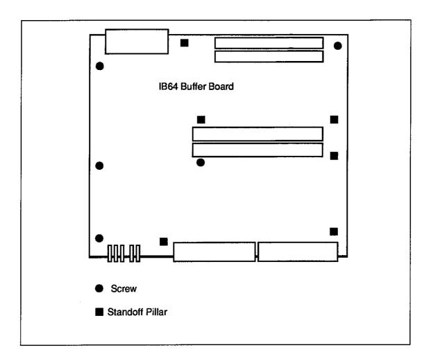
5. Remove the board by lifting so the Universal Module connectors are out of their hole in the case, and then sliding the board in the direction of the fan.
